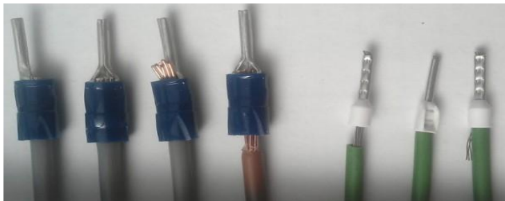
Terminal Crimps or Cable Lugs For Stranded conductors
